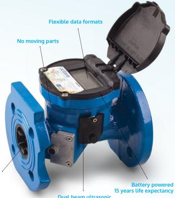
Dual beam ultrasonic technology for precise and ultra reliable metering
